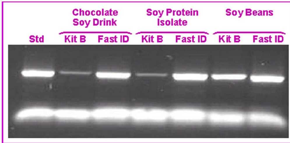
Figure 33.4. Comparison of Fast ID DNA extraction with a commercial kit – analysis by conventional PCR DNA was prepared from food samples using the Fast ID method and another commonly used DNA extraction kit. The quality of the DNA was assessed by conventional PCR. A standard amount of DNA (50 ng, quantified by absorbance at 260 nm) was introduced into each PCR reaction.
